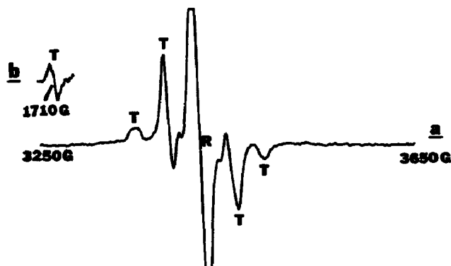
Figure 1. X-band ESR spectrum from photolysis of BAPA 1 at 77 K.
